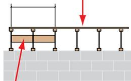
38x125mm min. timber blocks or BCI® blocking over min. 3 joists or 1.2m.
