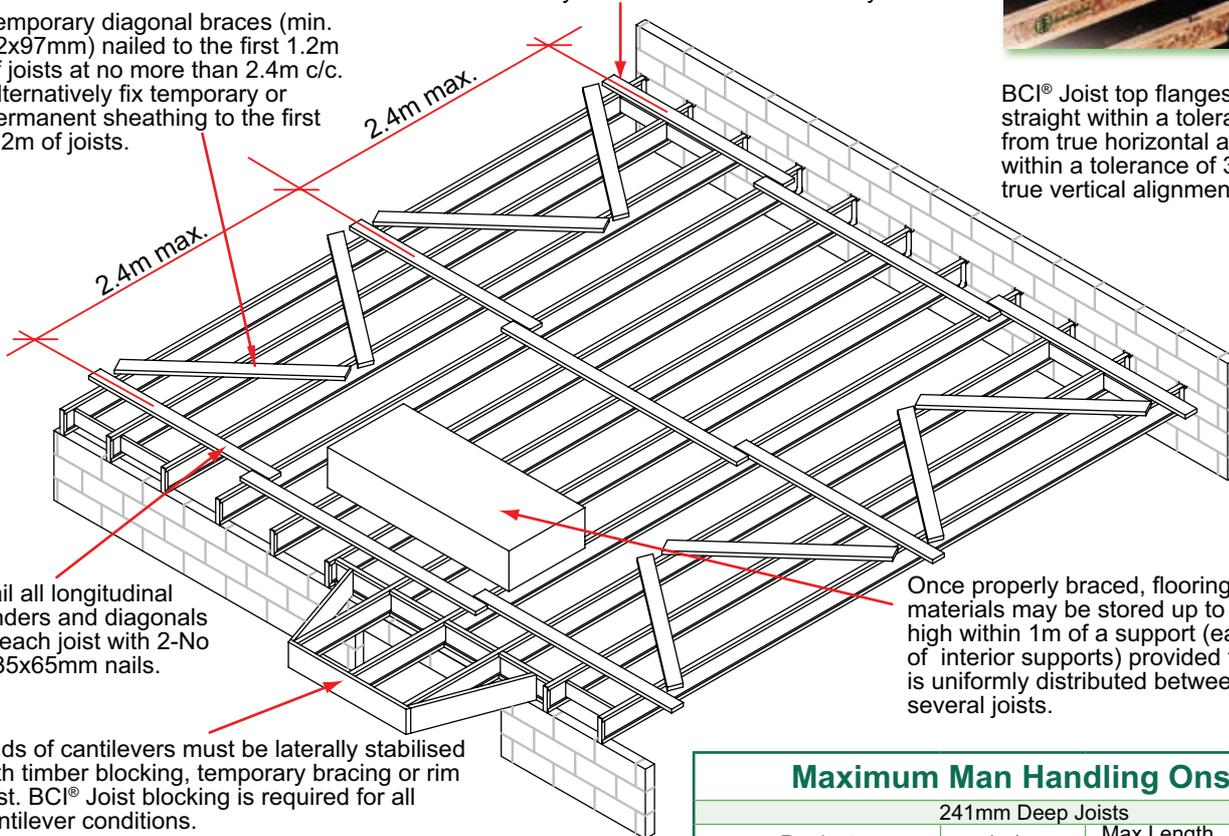
Once properly braced, flooring/ceiling materials may be stored up to 0.5m high within 1m of a support (each side of interior supports) provided the load is uniformly distributed between several joists.
